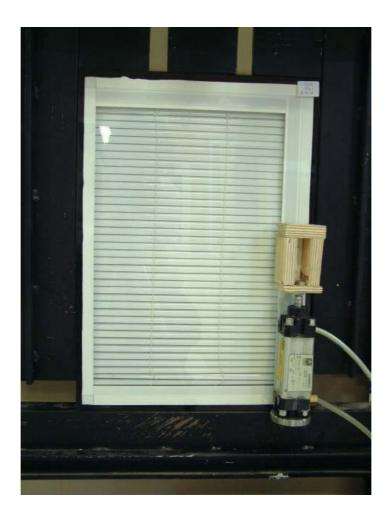
In this way, 100,000 opening and closing cycles were applied to the blind over its 80 mm run.
